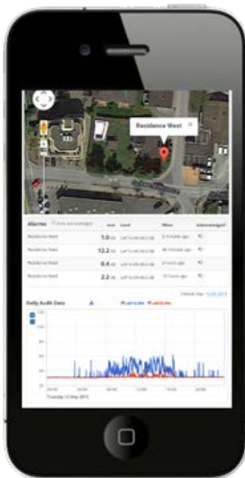
Live Noise Monitoring on the NoiseScout Web Portal with XL2 Sound Level Meter and NetBox
