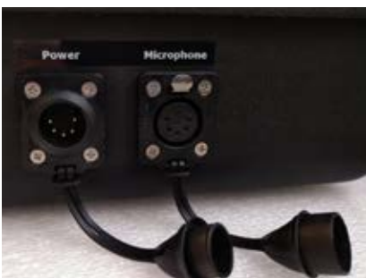
Removed protection plugs of waterproof connectors for microphone (IP63 configuration)
