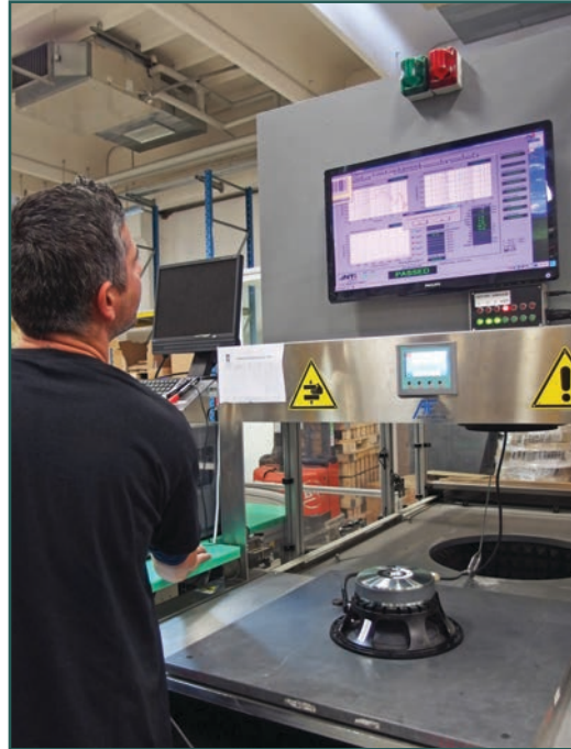
A factory worker at Eighteen Sound uses NTi Audio equipment during the QC stage.
